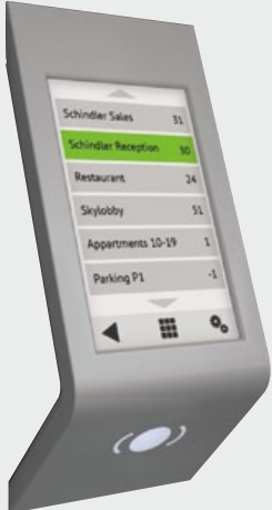
Touch-less operation If a card is held continuously at the PORT terminal, each authorized destination will be highlighted in turn, until the user makes his choice by removing his card.
